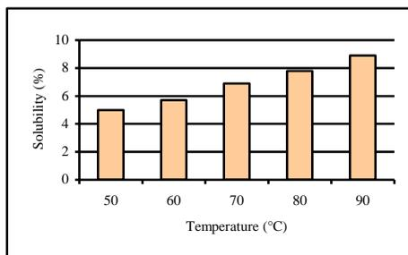
Fig. 7. Solubility of Rice Starch with Temperature
